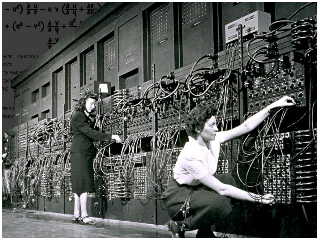
Fig. 7. Computer operators program the ENIAC, the first automatic, general-purpose, electronic, decimal, digital computer, by plugging and unplugging cables and adjusting switches (Source: History of computers )
